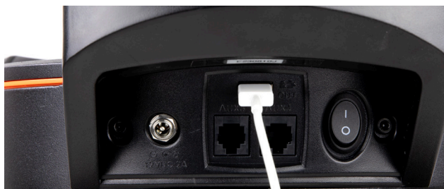
FIG 38: You can use the USB charging port on the Origin mount to charge your device in the field.
