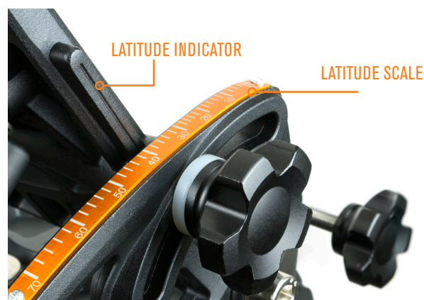
FIG D2: Turn the latitude adjustment knob on the wedge until the latitude indicator lines up with your current location's latitude on the scale.
