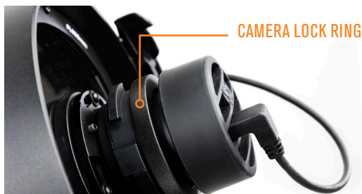
FIG 30: If you wish to rotate the camera orientation, first loosen the camera lock ring.
